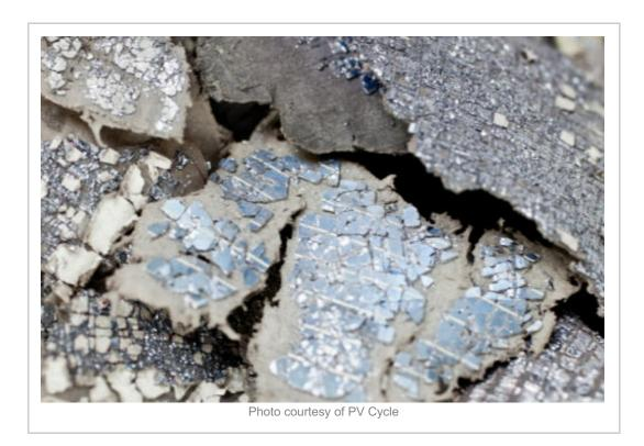
EPRI found that most panel recycling in Europe through the Waste Electrical and Electronic Equipment (WEEE) Directive—which established rules for solar panel recycling in 2012—happens at glass recyclers. Panels are crushed or shredded and then glass and metals are separated. Other chemical and thermal processes may be used to recover high-value material like silver or copper.
